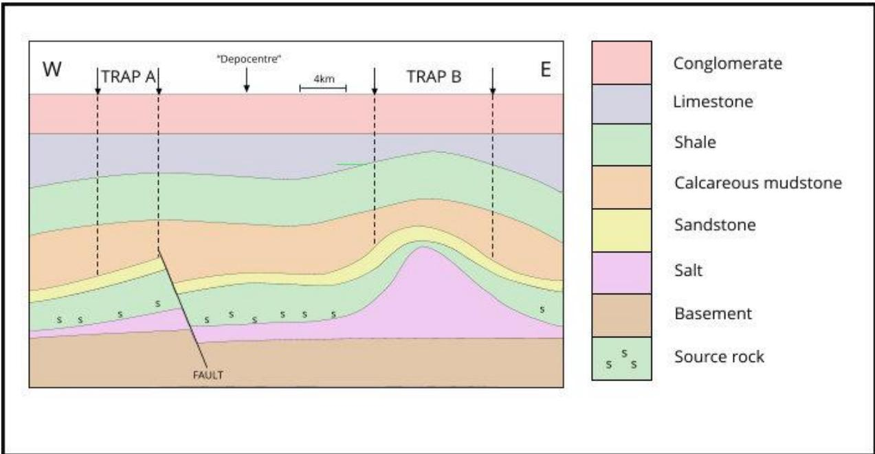
**Figure1 Geological cross section. (Note: In traps A & B the sandstone reservoir is sealed by calcareous mudstone)**
