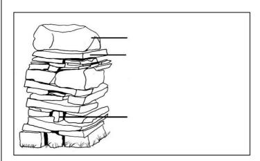
Narrower at the top, broader at the base, capstone, through stone, infill stone
