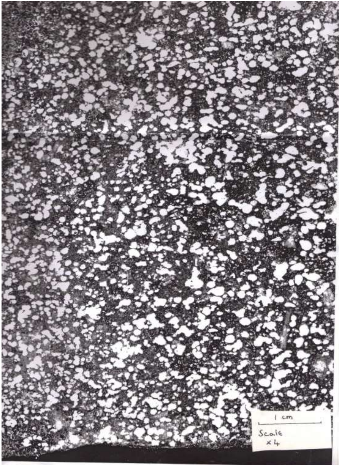
Photograph of a slice of vesicular basalt with the vesicles filled with Polyfiller. Enlarge to A4 size for point counting.
