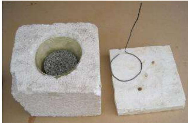
*Apparatus for determining specific heat showing inside*
