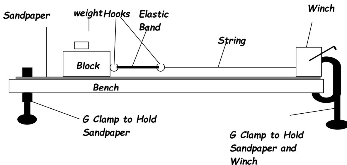
3. Set up the apparatus as in the diagram. Always use at least 500g weight on the blocks. Use bluetack to hold a 1m strip of till roll paper along the side of the long piece of sand paper.
