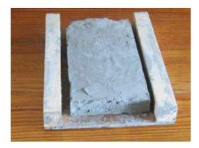
Porosity of rock samples E P F 15 min per rock Students measure the porosity of irregularly shaped samples. First the volume must be found by weighing the sample in air and in water. The sample is soaked for 24 hours and weighed again in air. The change in weight in grams is the weight of the water absorbed in and this equals the volume of the pores in cc. A series of samples can be measured, for instance, sandstones of different ages or different types of limestone.
